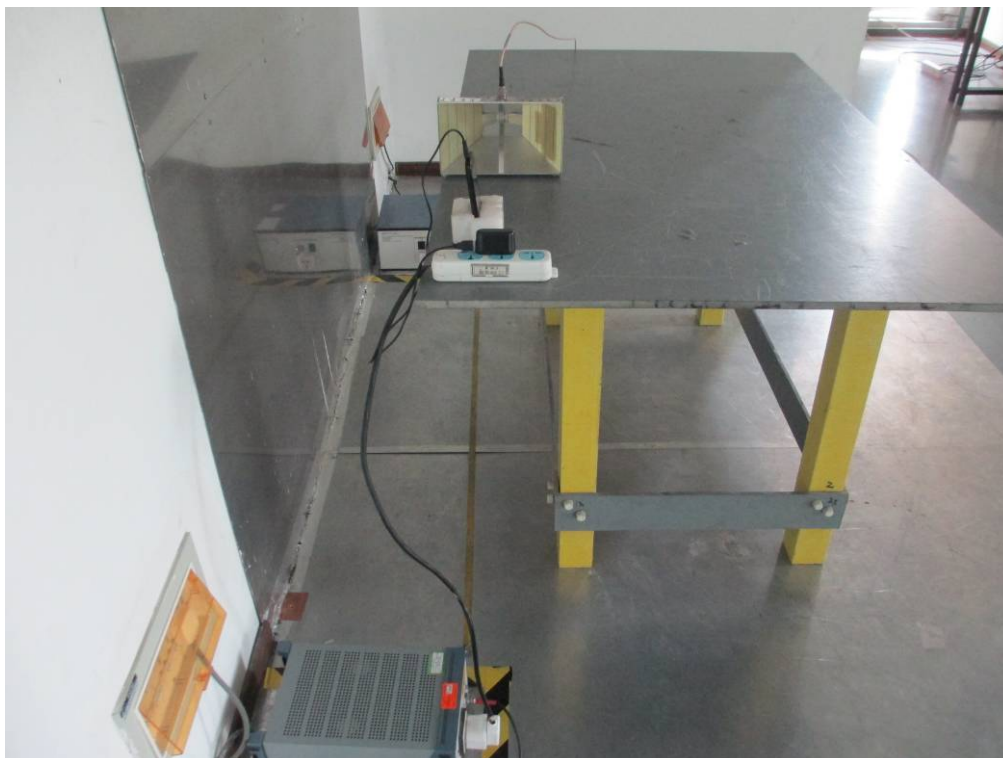
Conducted Emissions Test Setup Side View
