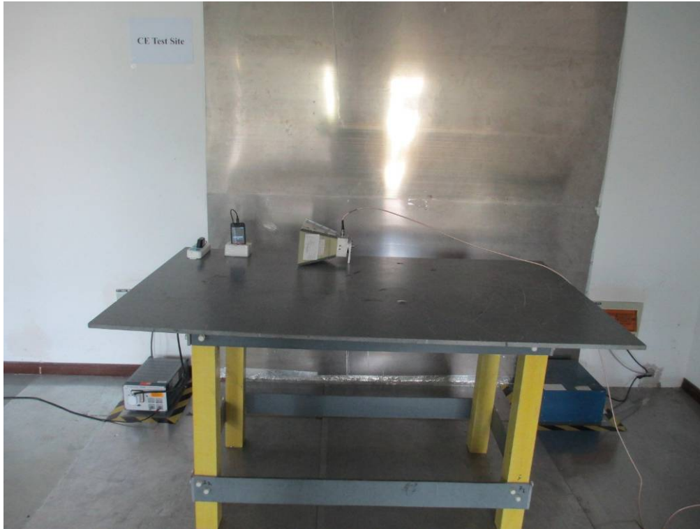
Conducted Emissions Test Setup Front View
