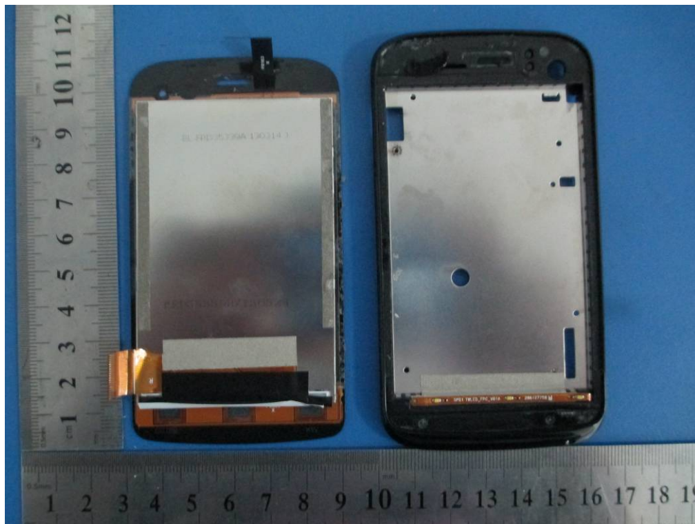
Uncover LCD - Top View
