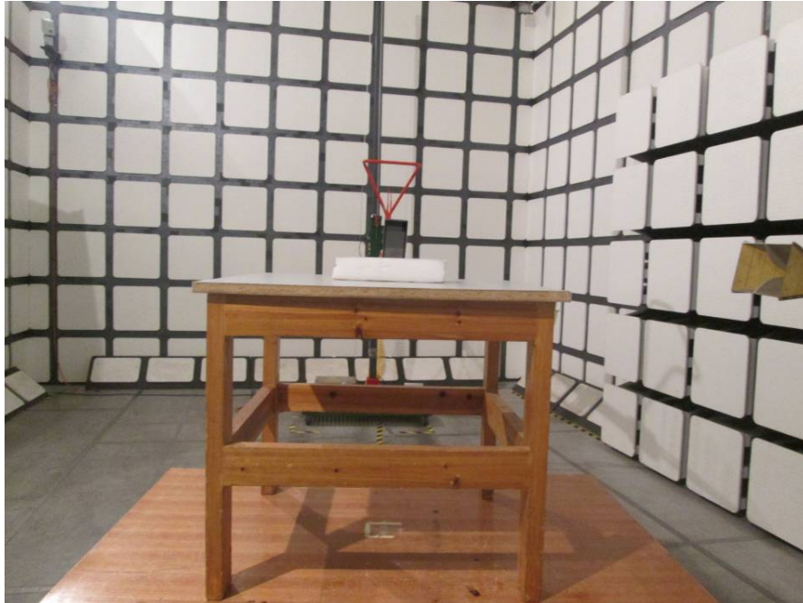
Radiated Emissions Test View (Below 1 GHz)
