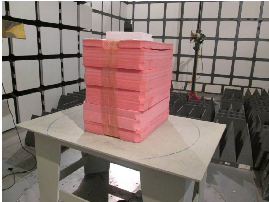
Radiated Emissions Test View (Above 1 GHz)
