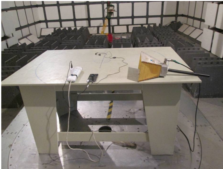
Radiated Emissions Rear View (Above 1GHz)
