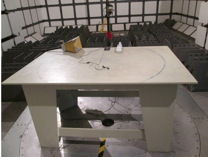
Radiated Emissions Front View (Above 1GHz)
