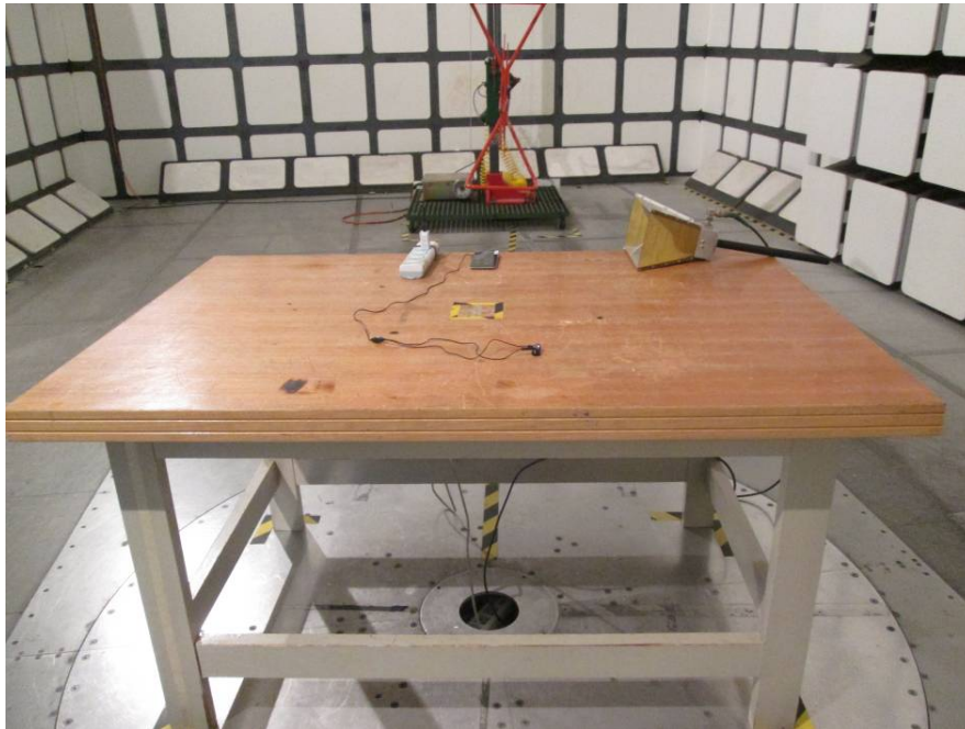
Radiated Emissions Front View (Below 1GHz)
