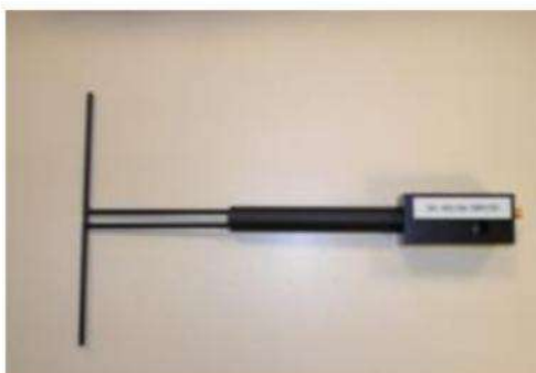
Figure 1 – Satimo COMOSAR Validation Dipole
