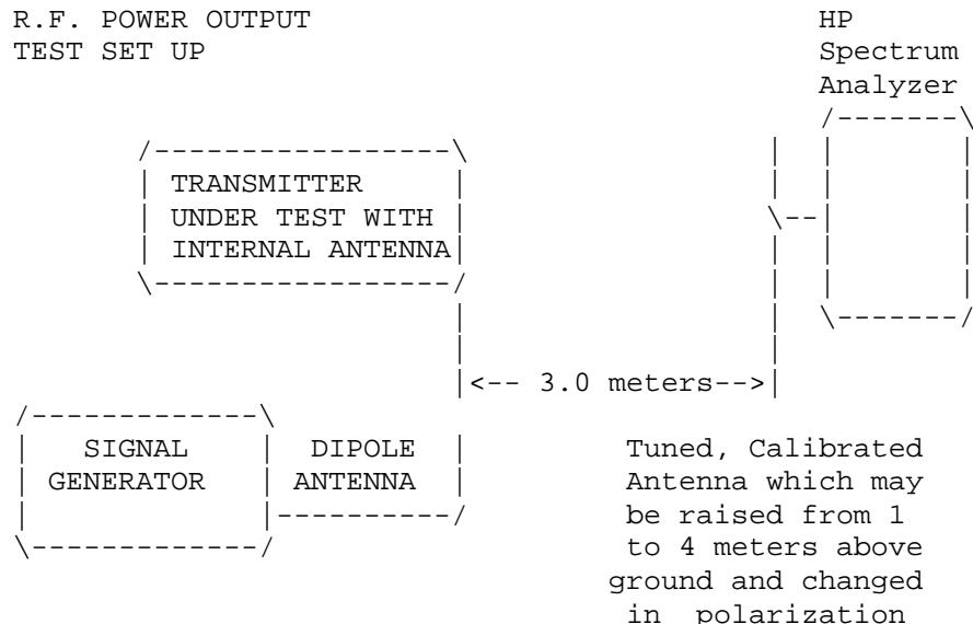
Equipment placed 1 meter above ground
