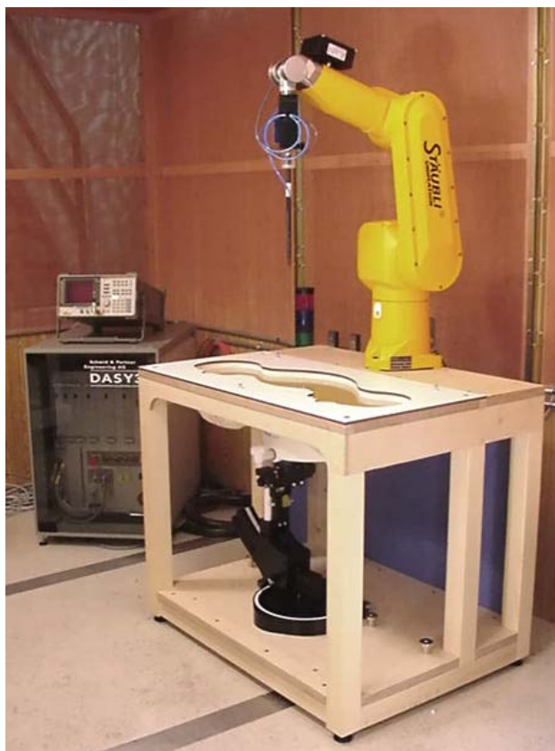
DASY3 SAR Measurement System with SAM Phantom
