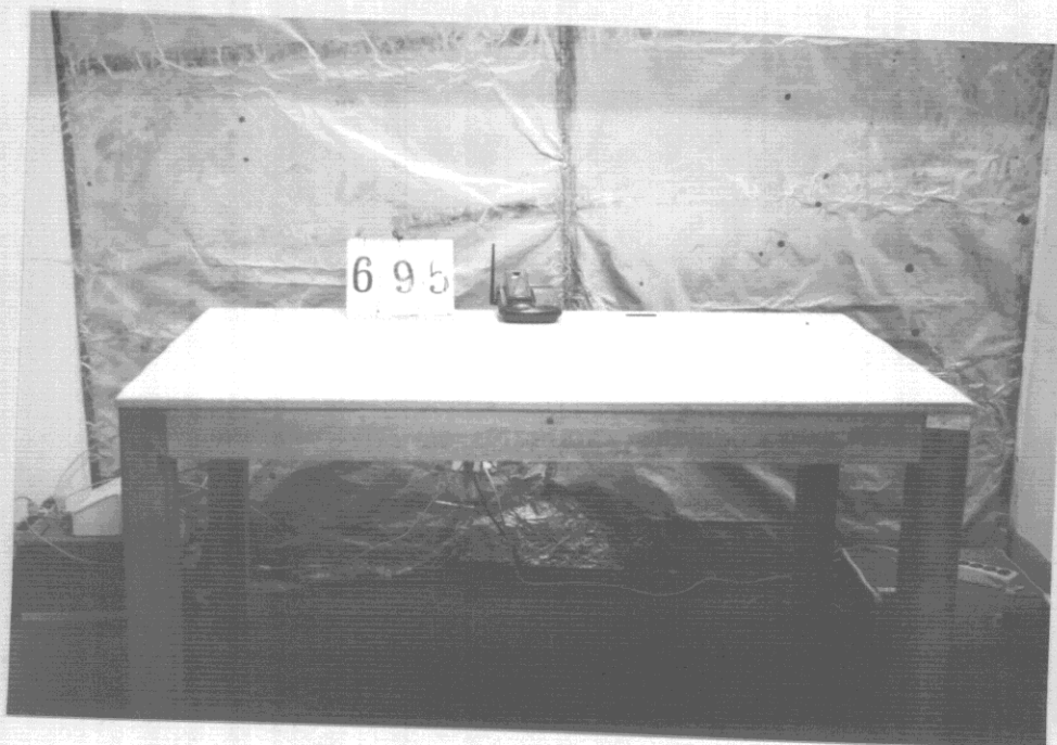
Fig. 3 Conducted emissions test placement (idle only)
