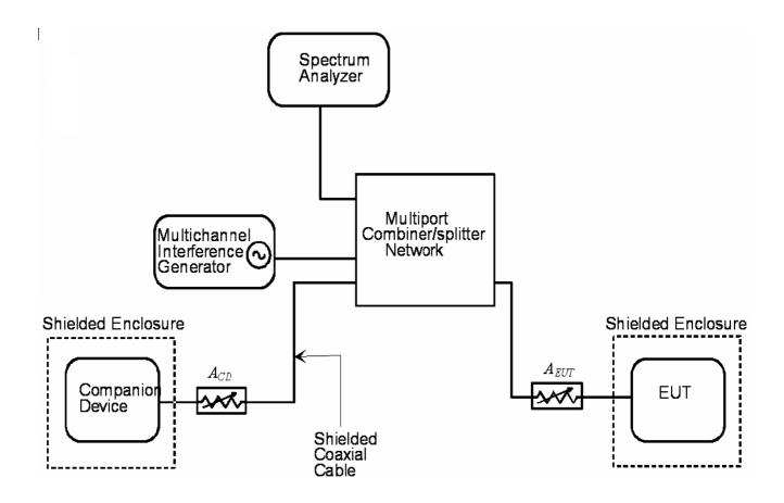
**Test Set-Up 1**
