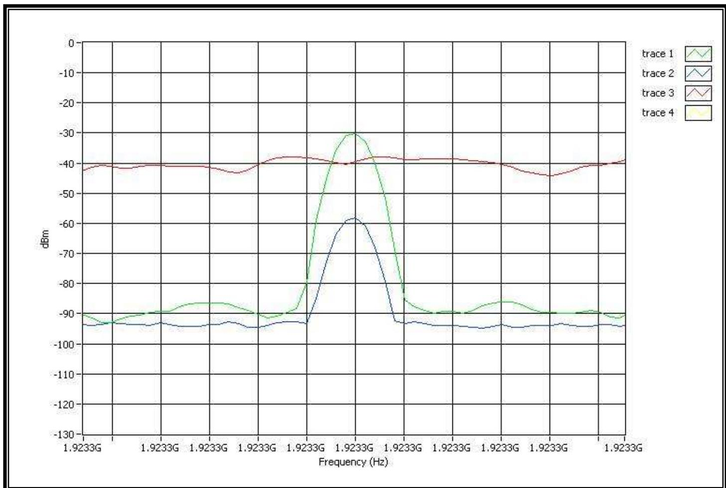
Note1: Trace1 (green) is the interference on all 5 carriers. The level is  $T_u+U_m+10$ dB.
