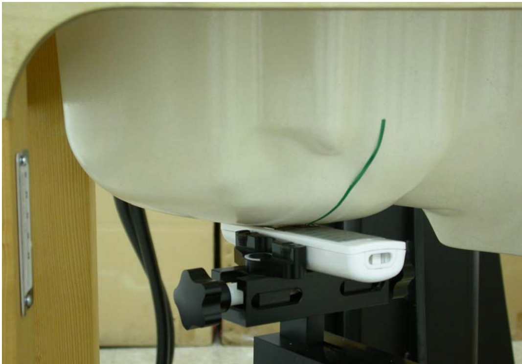
Measurement Position of Right-Cheek (RC) with Handset
