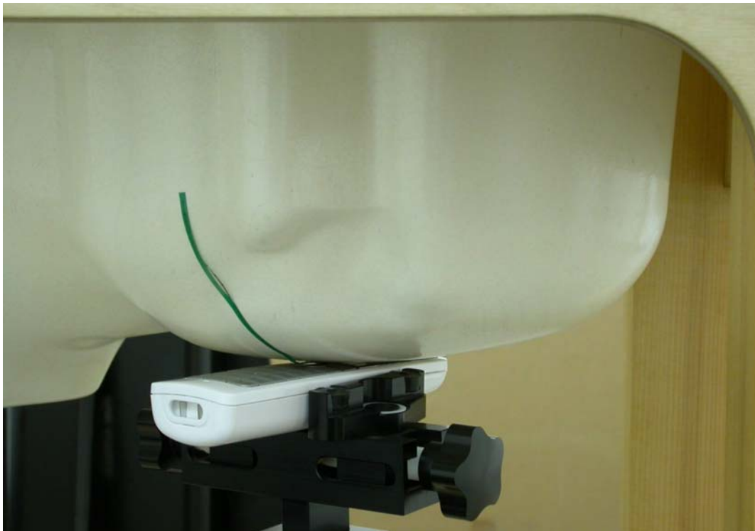
Measurement Position of Left-Cheek (LC) with Handset
