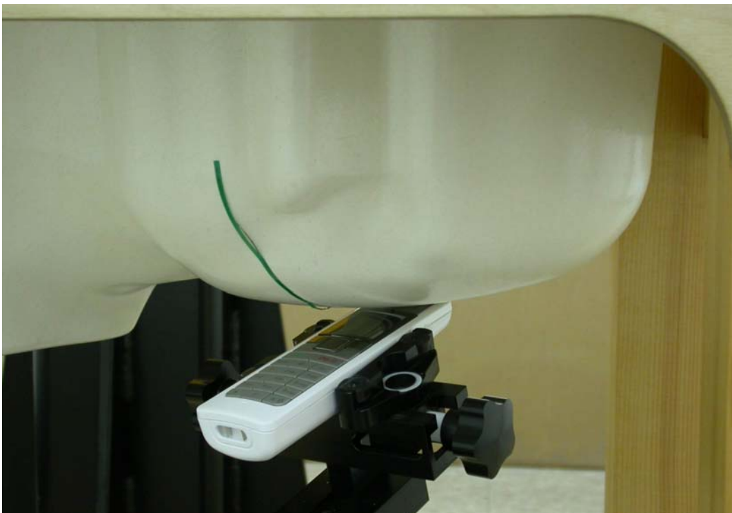
Measurement Position of Left-Tilt (LT) with Handset
