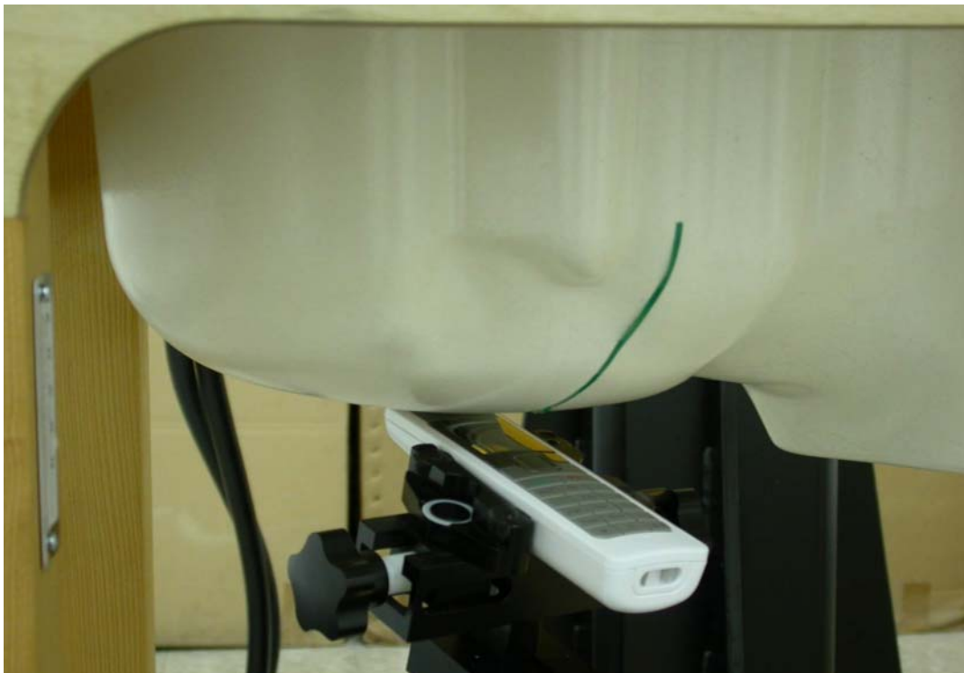
Measurement Position of Right-Tilt (RT) with Handset
