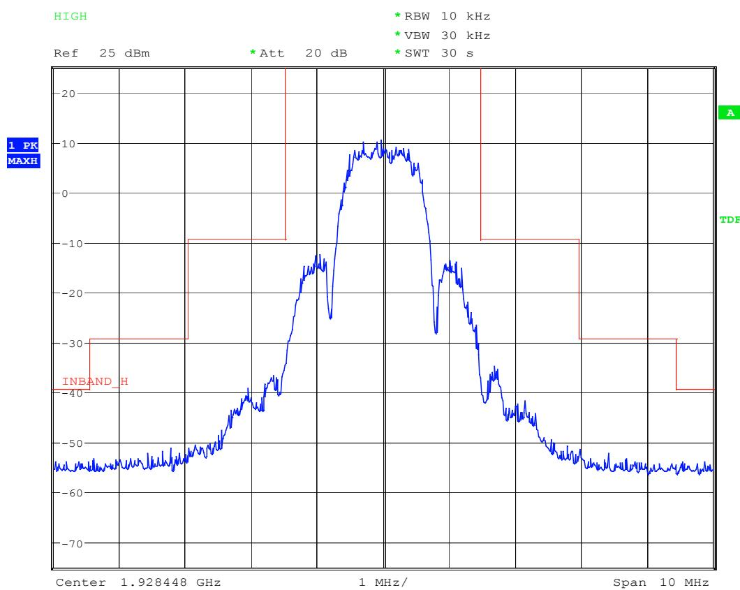
**Out-of-band Unwanted Emission:****a) CH FL****Out-of-band Unwanted Emissions (below 1GHz): CH FL**
