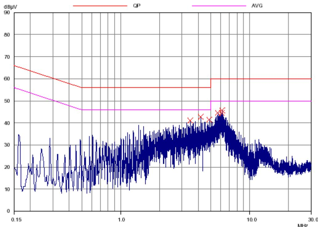
Operation Mode : Base Unit ChargingTest Date : Jun. 21, 2007 Temperature : 22 °C Humidity : 54 %Mode: Base Unit Charging
