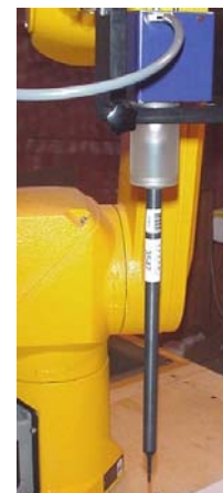
EX3DV4 E-Field Probe
