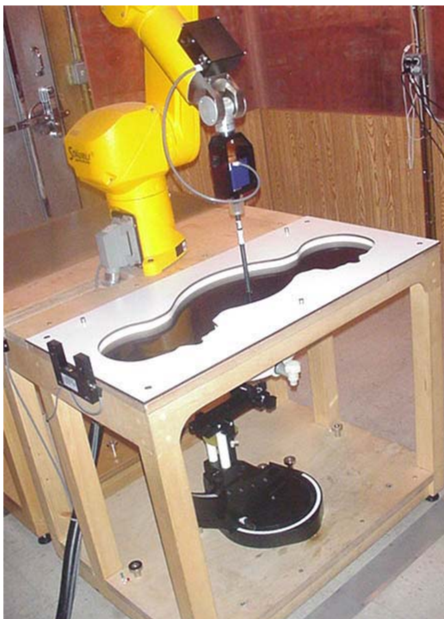
DASY4 SAR Measurement System with SAM phantom and 5GHz Fluid
