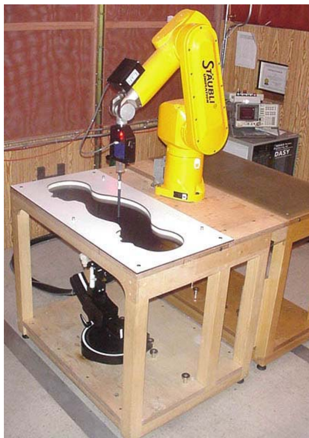
DASY4 Measurement System with SAM Phantom and 5GHz Fluid
