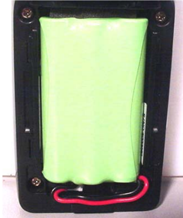
DUT with NiMH Battery 3.6 V, 800 mAh
