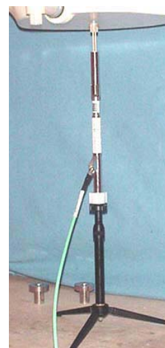
5 GHz Dipole Setup
