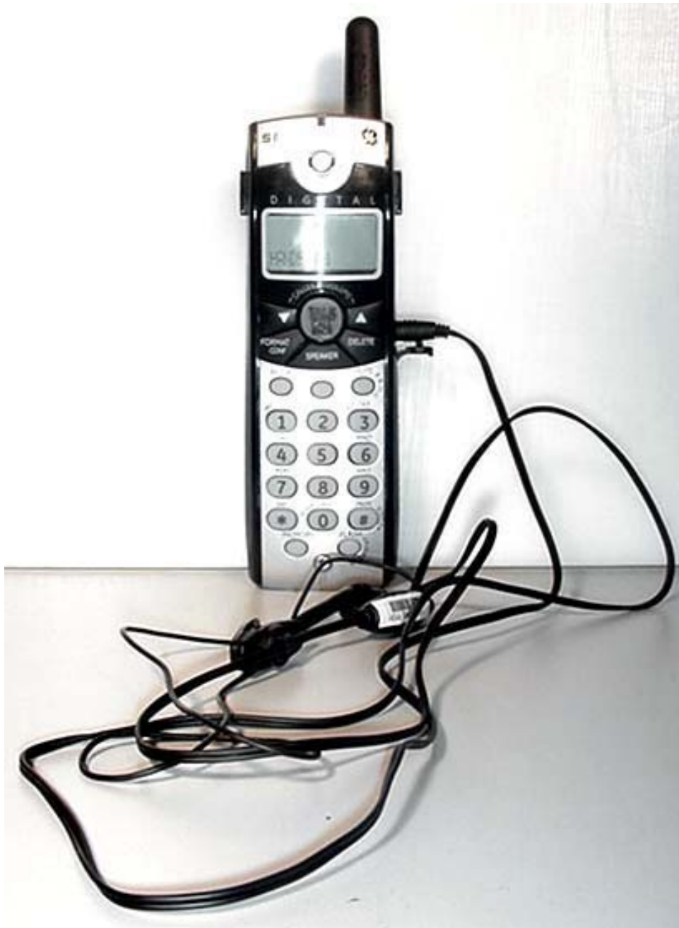
DUT with Generic Ear-Microphone Accessory
