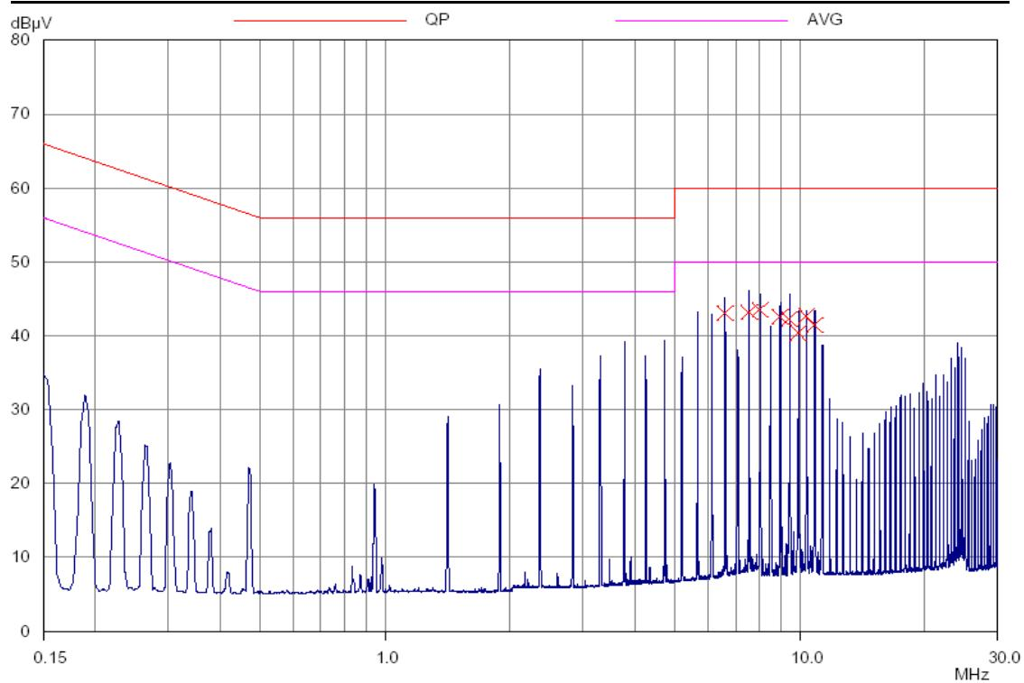
Operation Mode : Base On Line NeutralTest Date : Feb. 15, 2008 Temperature : 17 °C Humidity : 62 %
