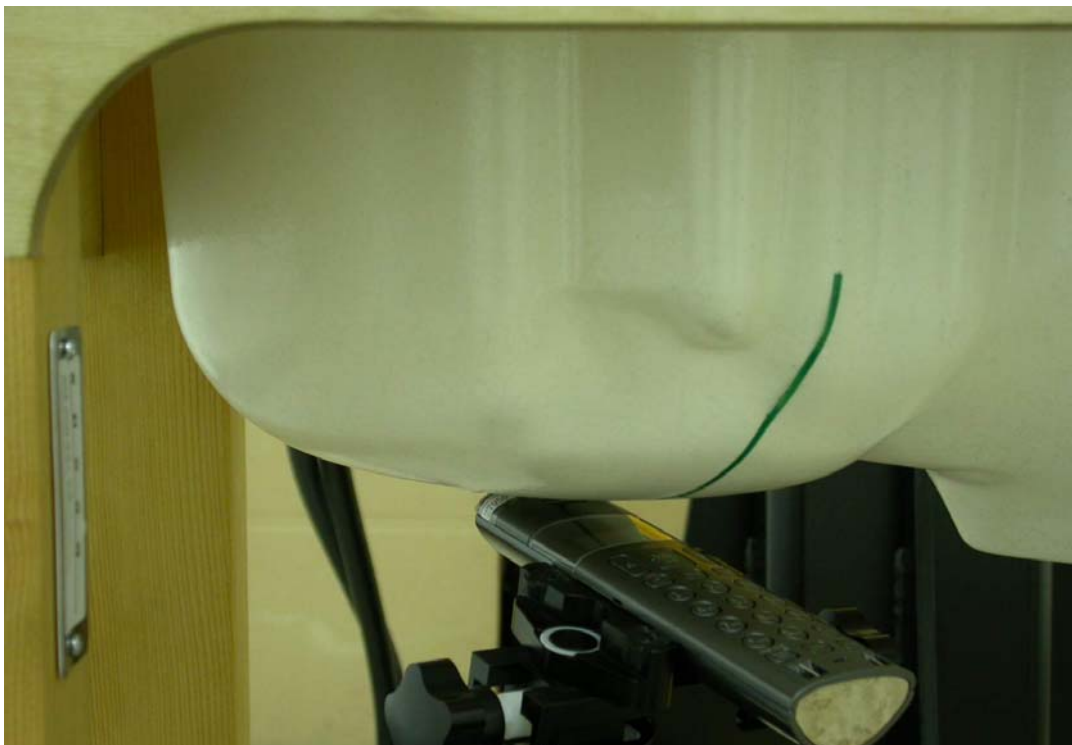
Measurement Position of Right-Tilt (RT) with Handset
