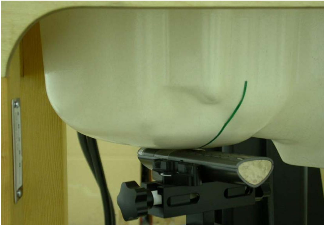
Measurement Position of Right-Cheek (RC) with Handset
