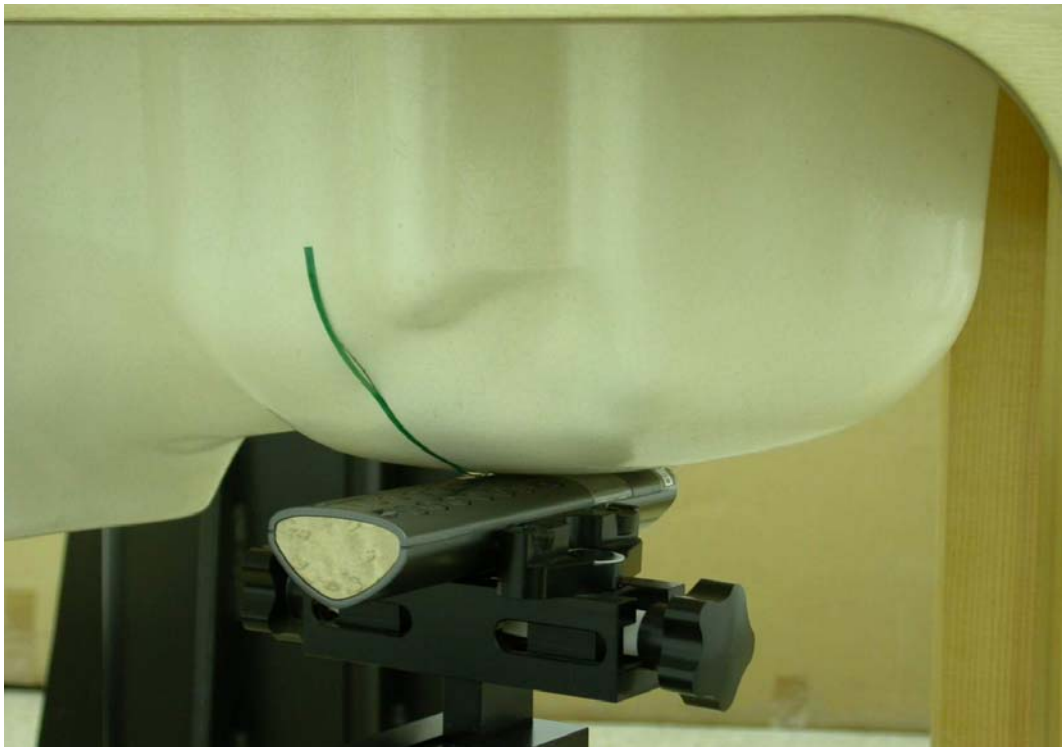
Measurement Position of Left-Cheek (LC) with Handset
