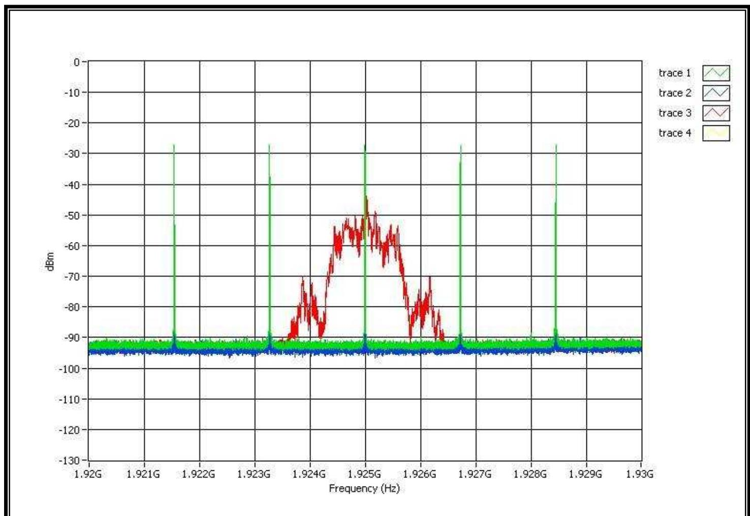
Note1: Trace1 (green) is the interference on all 5 carriers. The level is  $T_u+U_m+10\text{dB}$ .
