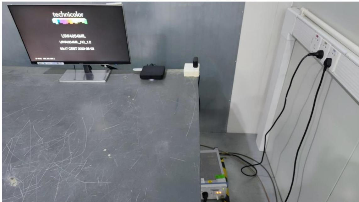
**Radiated Emissions Test Photos****9 kHz to 30 MHz**
