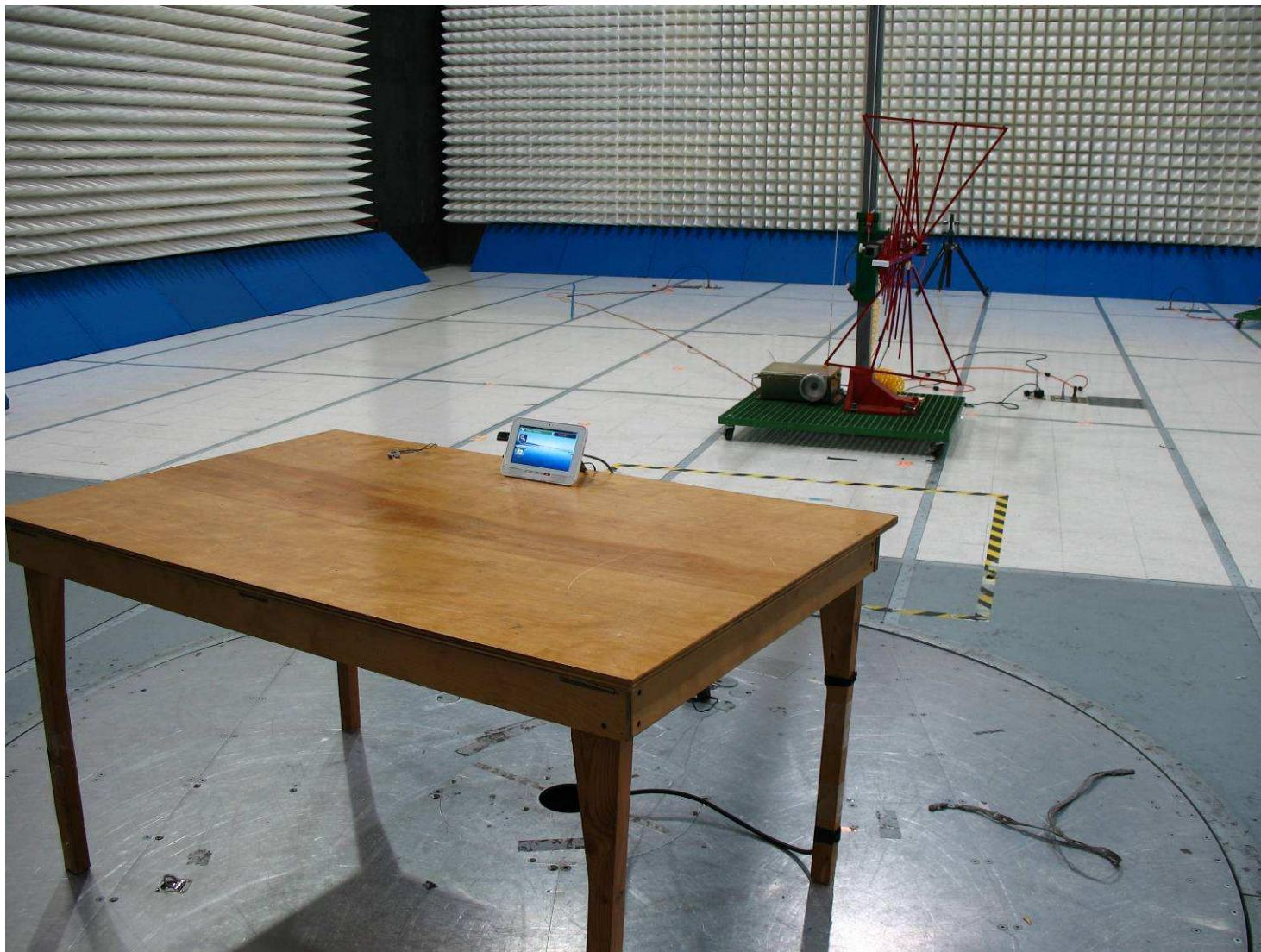
Part 22/24 Radiated Tests
