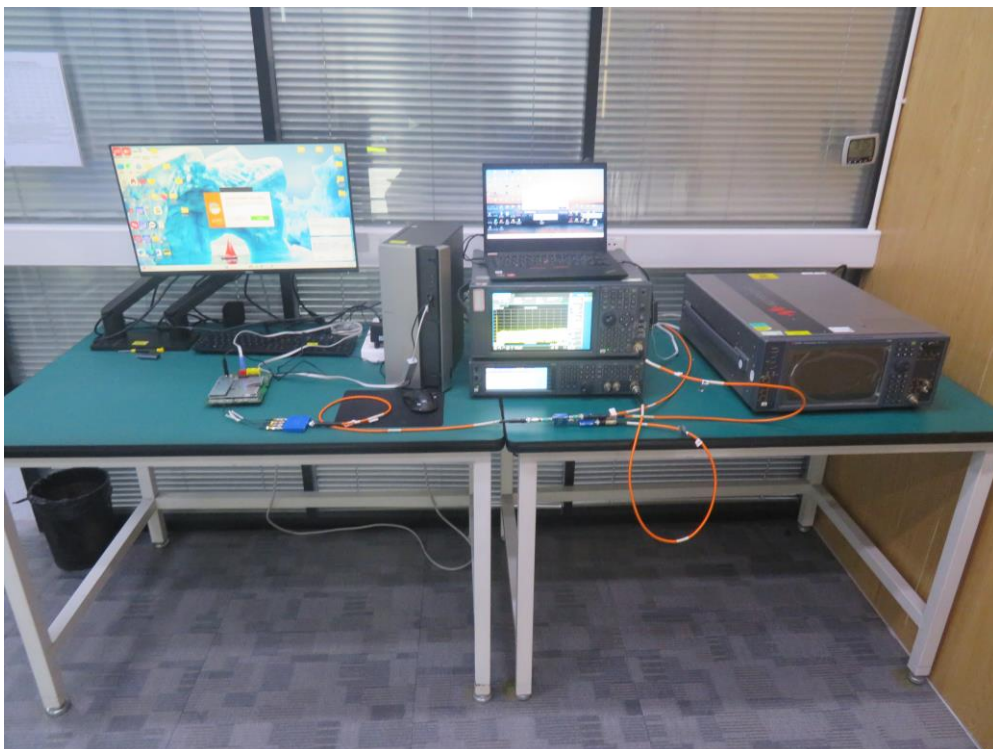
Description: Dynamic Frequency Selection Test Setup
