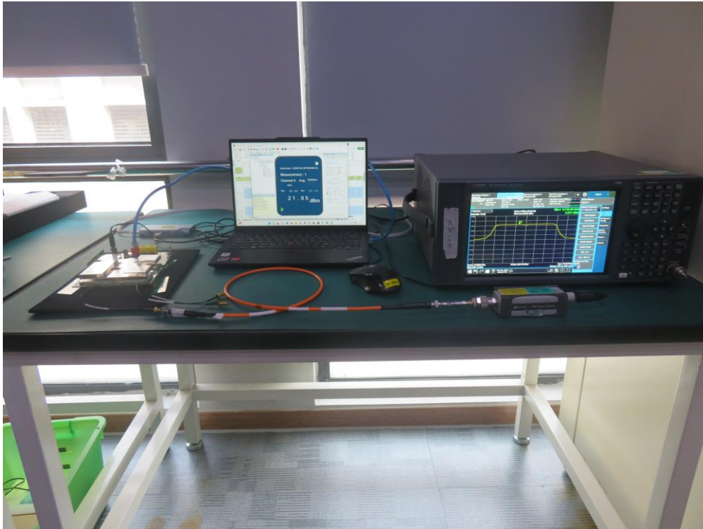
Description: Dynamic Frequency Selection Test Setup
