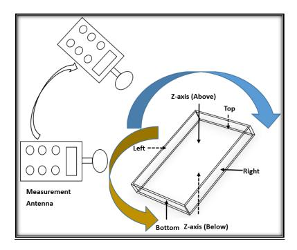
Note: The measurement antenna are moving and surrounding the EUT when performed the test, the test results recorded the highest values for each sides of the EUT (left/right/top/bottom/z-axis)
