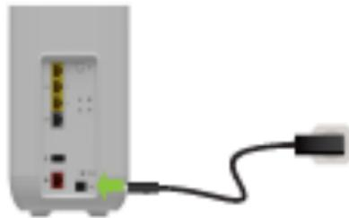
Plug the connector of the electric power supply adapter into the power inlet port of your Ethernet gateway. Plug the adapter into a nearby power outlet.
