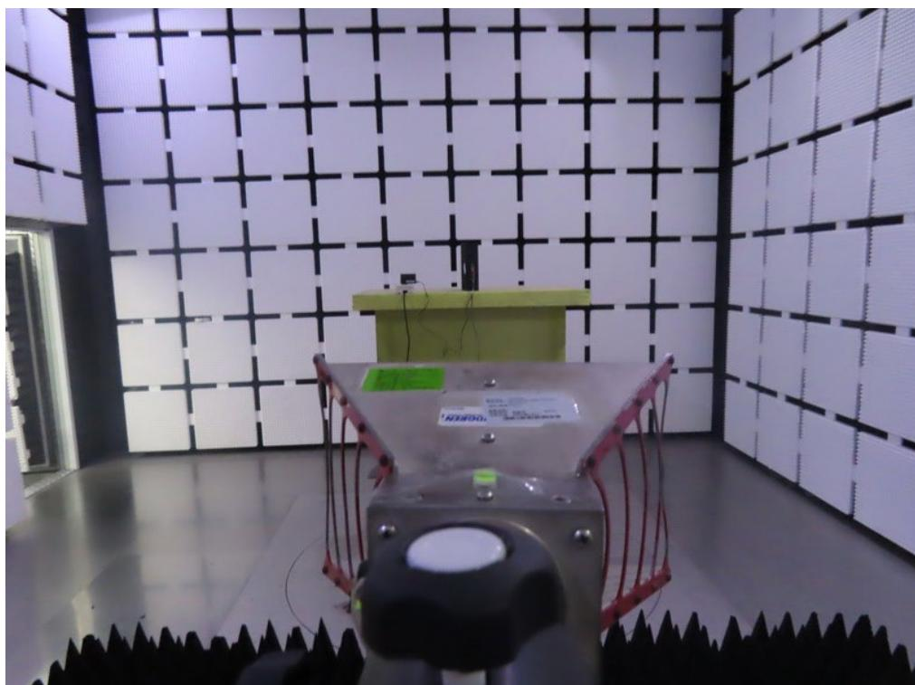
**Radiated Emissions Test Photos****Above 18 GHz**
