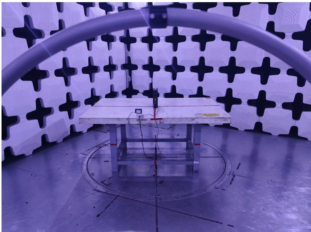
**Radiated Emissions Test Photos****30 MHz to 1 GHz**
