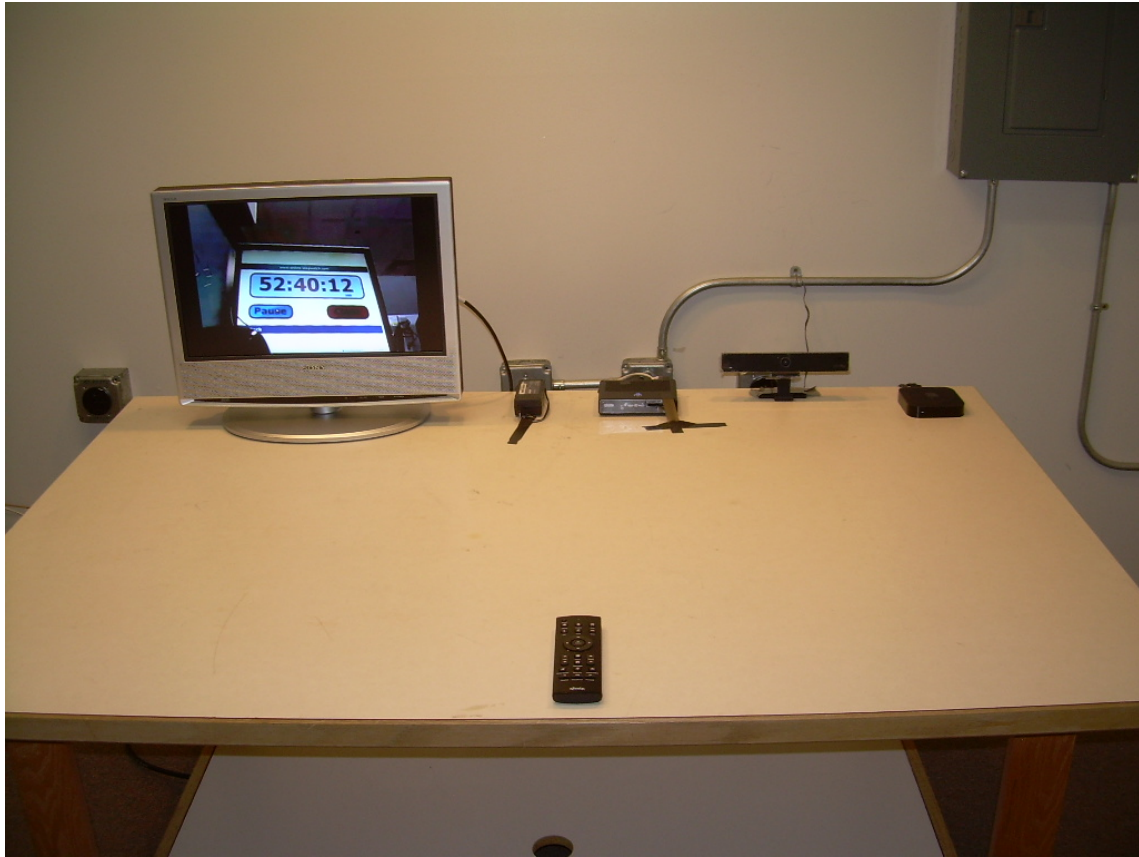
Front View Conducted Disturbance Test Configuration
