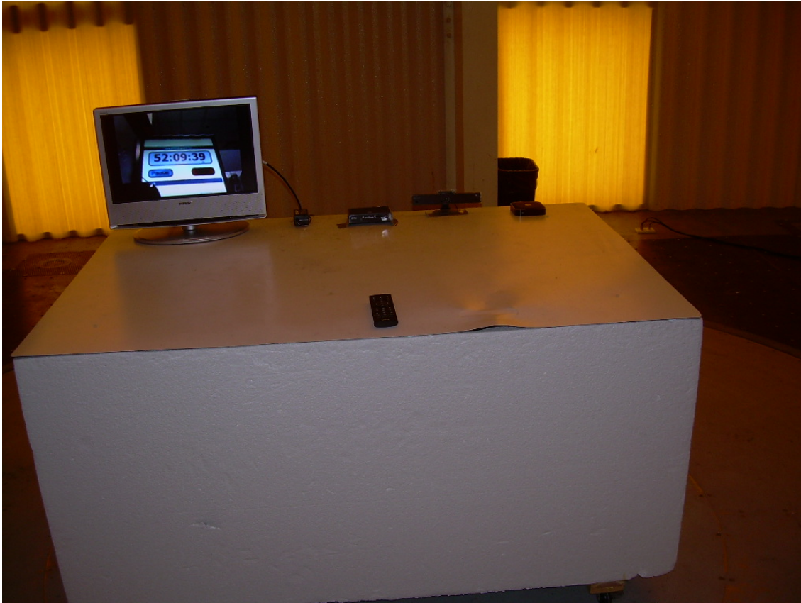
Front View Radiated Disturbance Test Configuration
