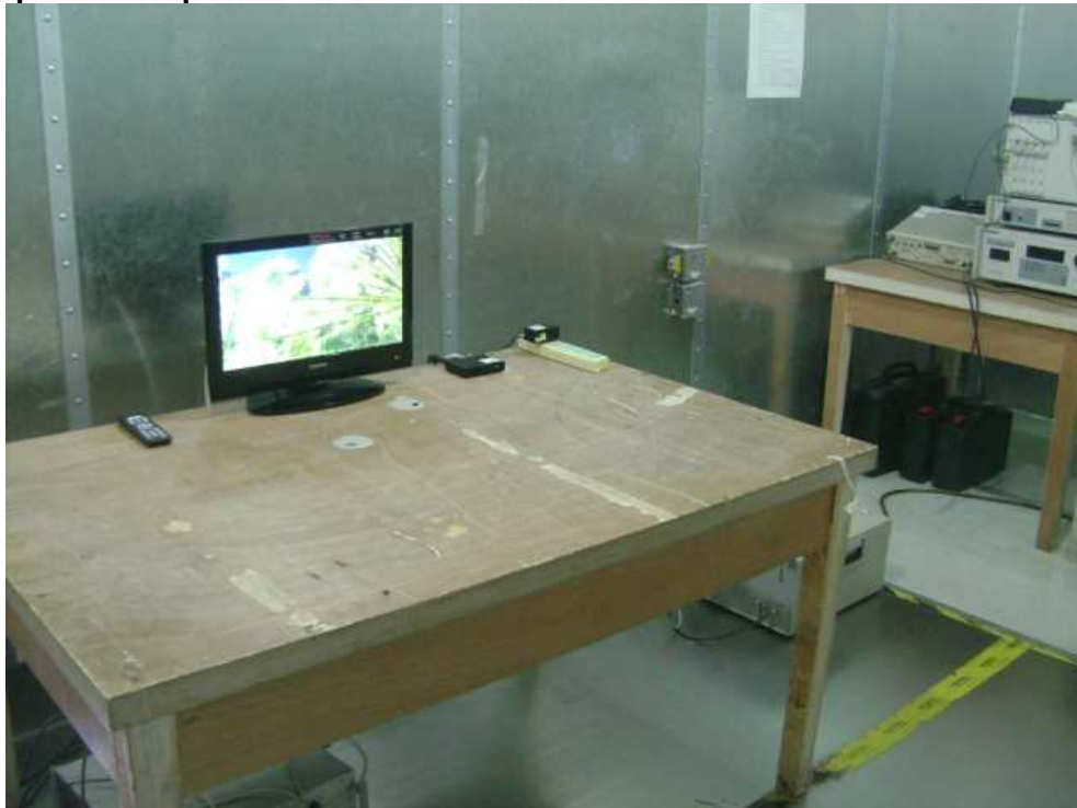
Photograph 2: Set-up for Spurious Emissions 30MHz – 1GHz
