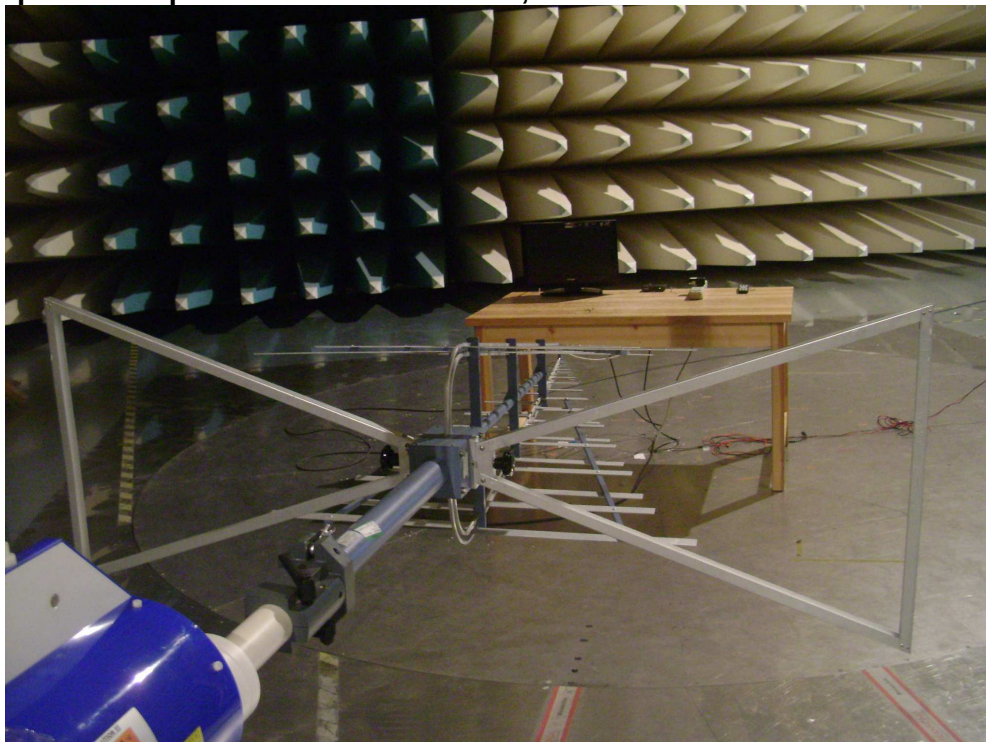
Photograph 2: Set-up for Radiated Emissions, 30MHz-1GHz
