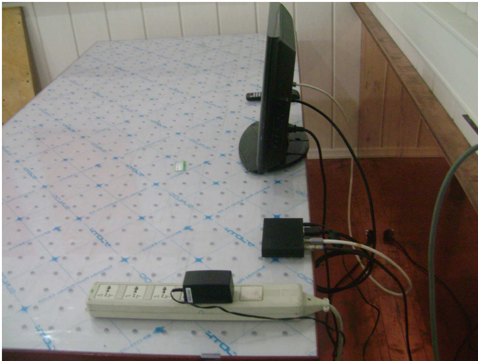
Photograph 2: Set-up for Radiated Emissions, 30MHz-1GHz
