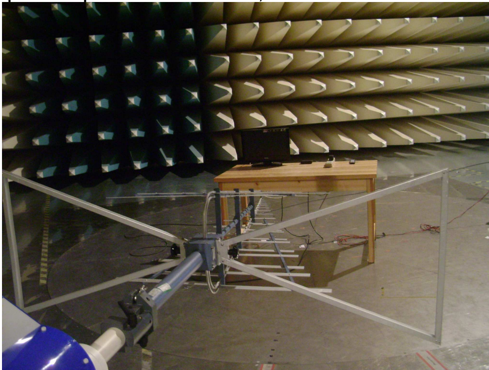
Photograph 2: Set-up for Radiated Emissions, 30MHz-1GHz
