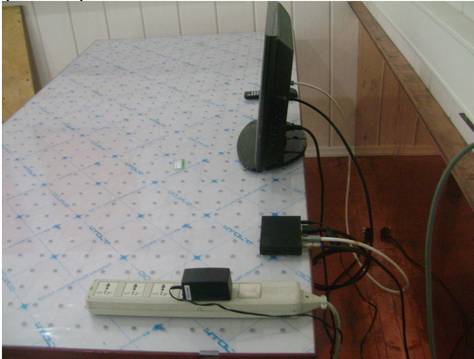
Photograph 2: Set-up for Radiated Emissions, 30MHz-1GHz
