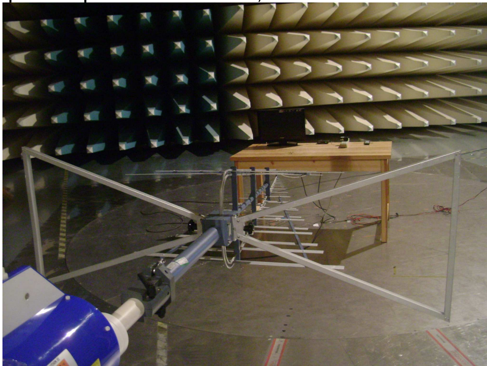
Photograph 2: Set-up for Radiated Emissions, 30MHz-1GHz
