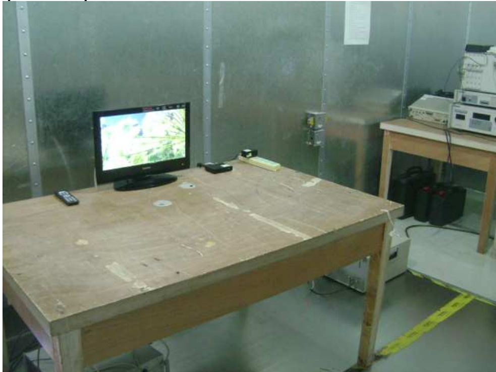
Photograph 2: Set-up for Radiated Emissions, 30MHz-1GHz
