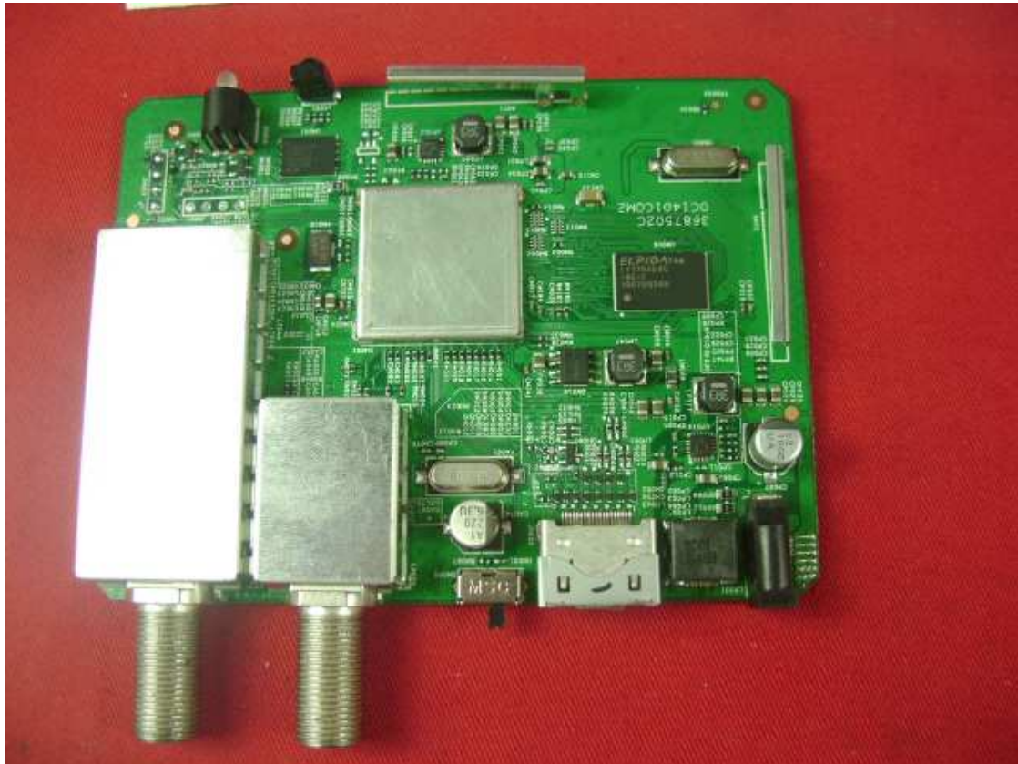
Pic5: PCB component side (with shielding) of DCI401COM2
