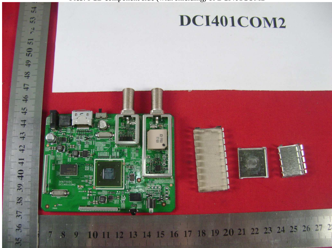
Pic6: PCB component side (without shielding) of DCI401COM2
