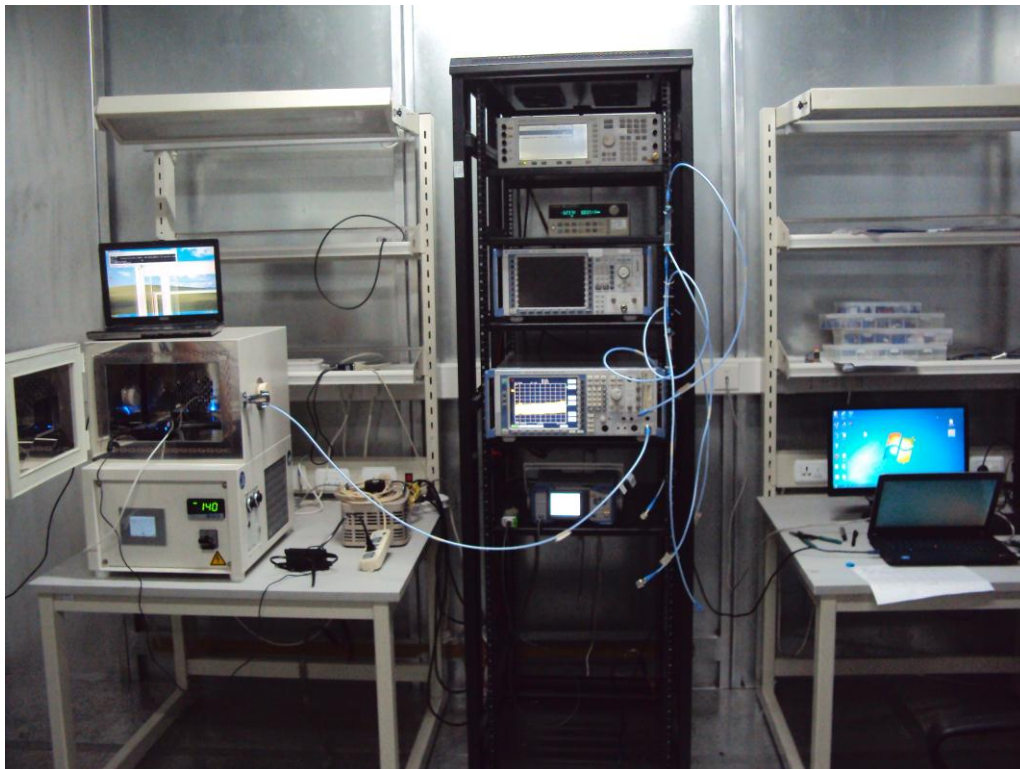
Photograph 4: Set-up for Conducted emission
