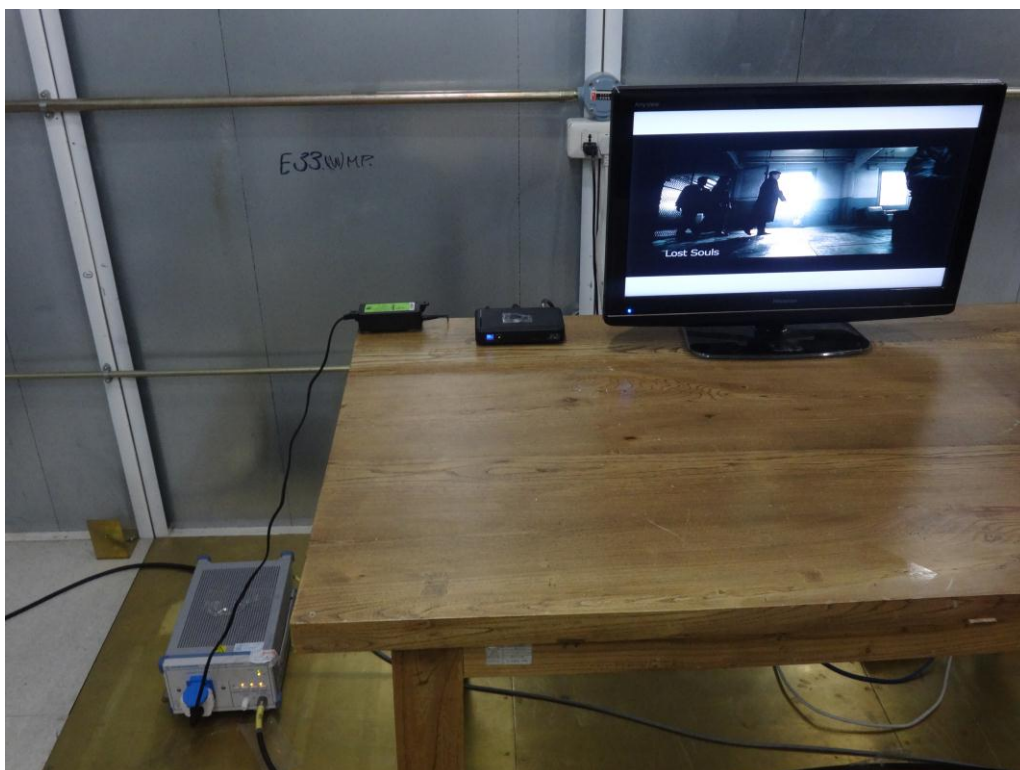
Photograph 4: Set-up for Conducted emission
