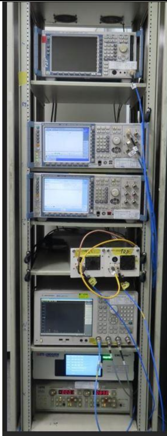
Fig.2 Test Chamber – Network Analyzer
