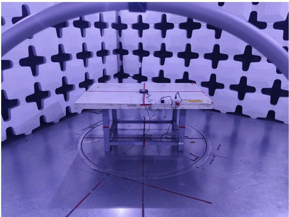
**Radiated Emissions Test Photos****30 MHz to 1000 MHz**
