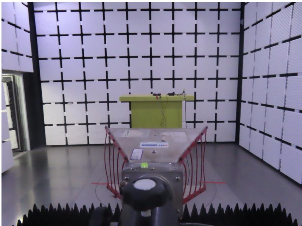
**Radiated Emissions Test Photos****Harmonic(18 GHz to 26.5 GHz)**
