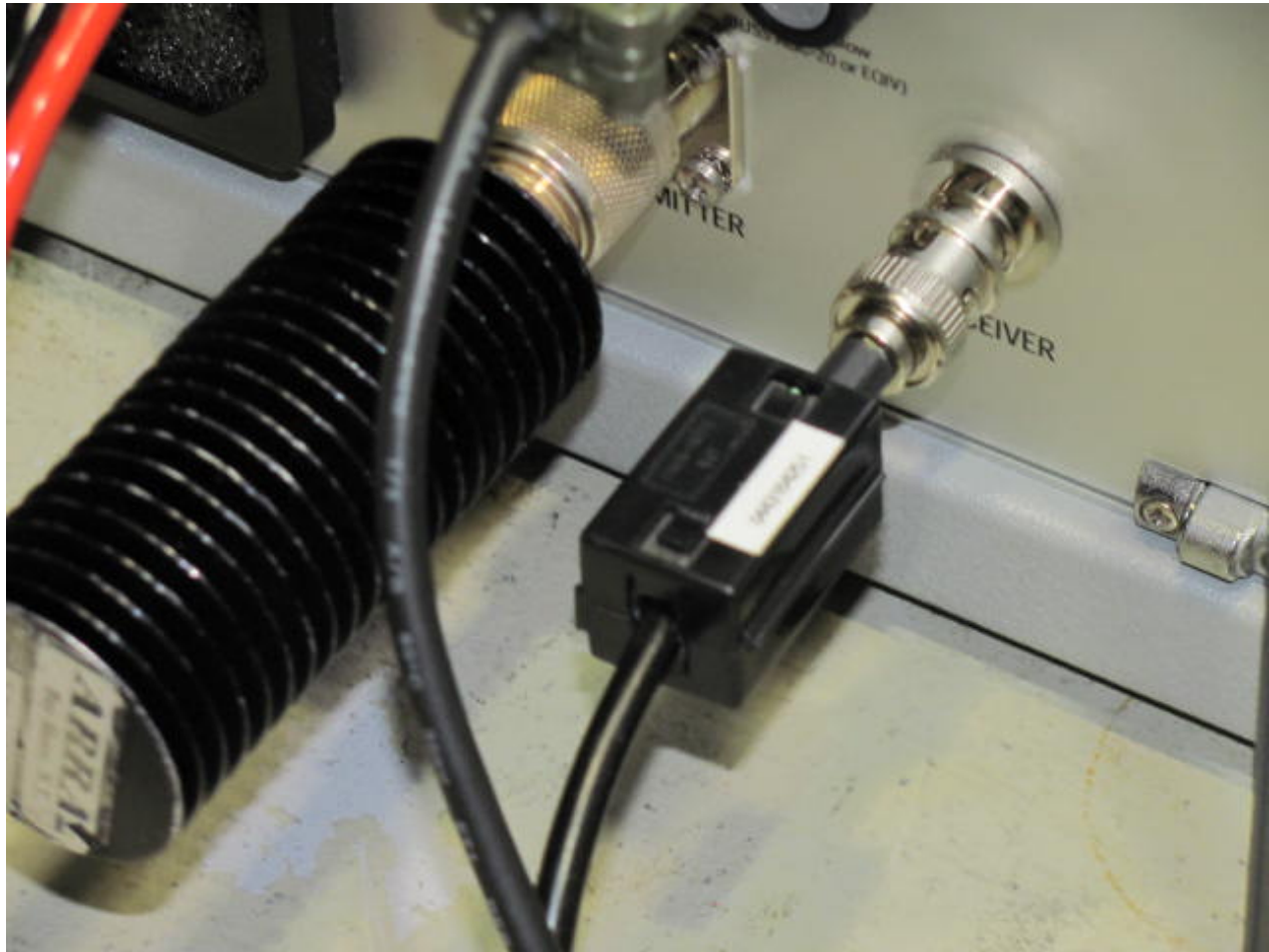
Figure 3 showing module connection to Antenna Isolation Board
