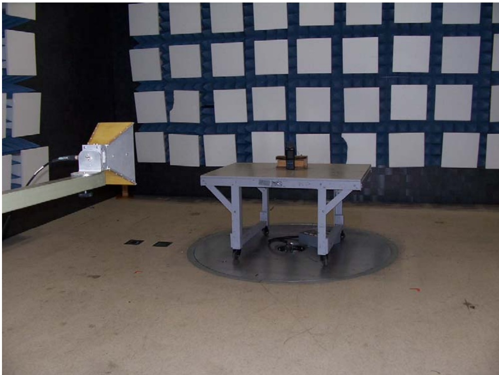
Figure 4: Spurious Radiated Emissions 1 GHz to 10 GHz Setup
