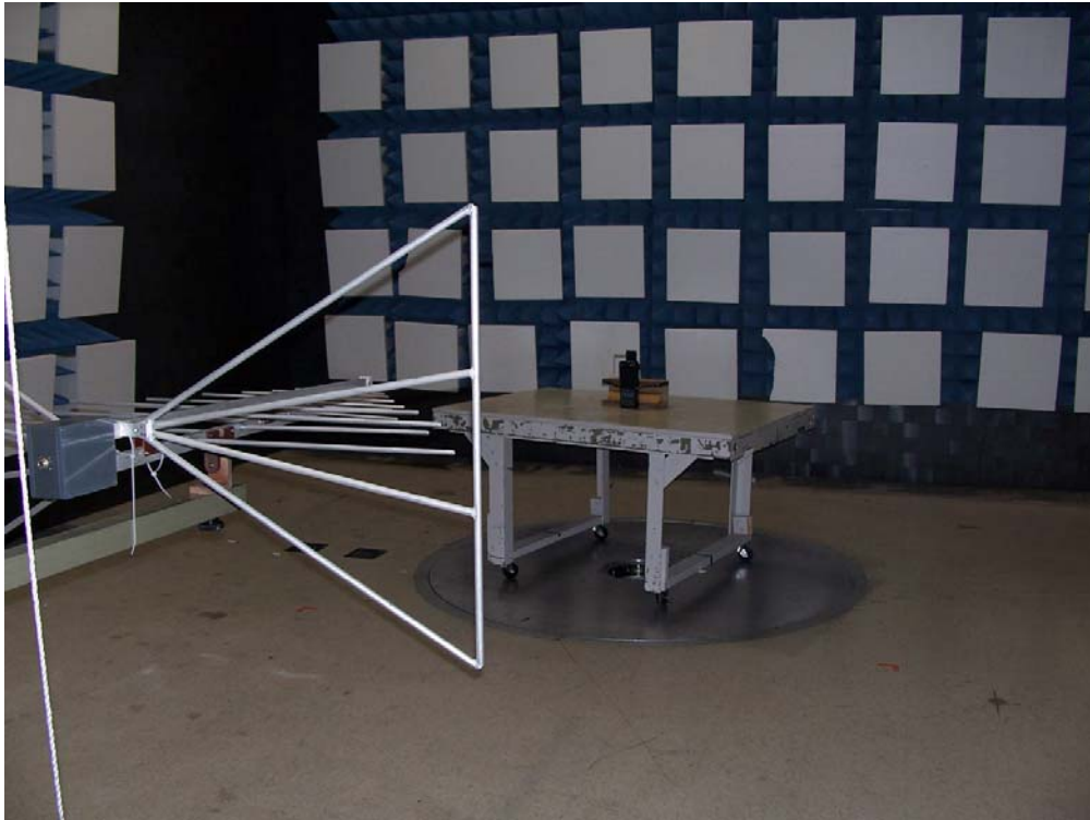
Figure 3: Radiated Emissions 30 MHz to 1 GHz Setup
