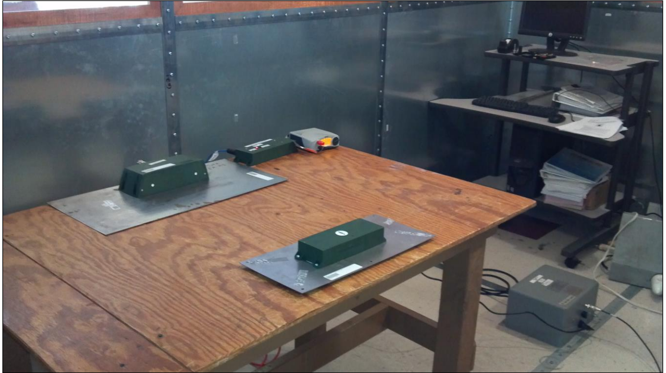
Photograph 3. Conducted Emissions, 15.207(a), Test Setup
