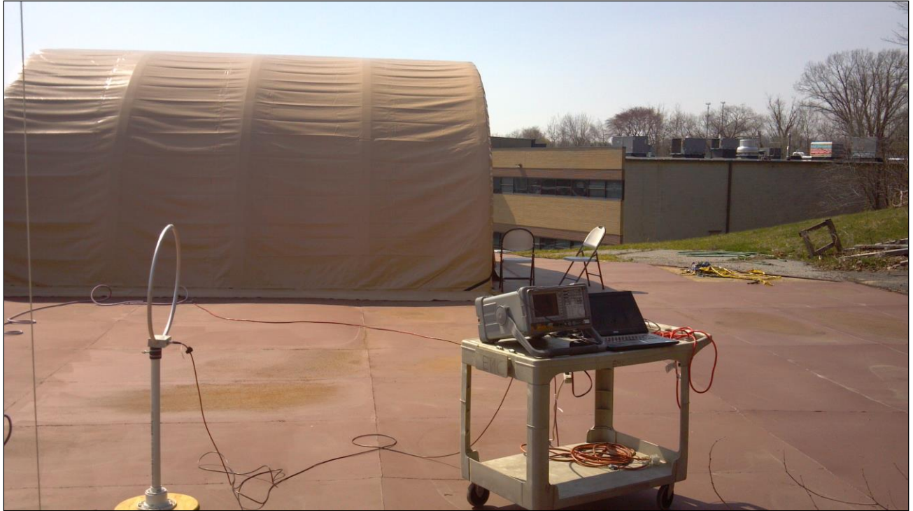
Photograph 6. Radiated Spurious Emissions, Test Setup, OATS
