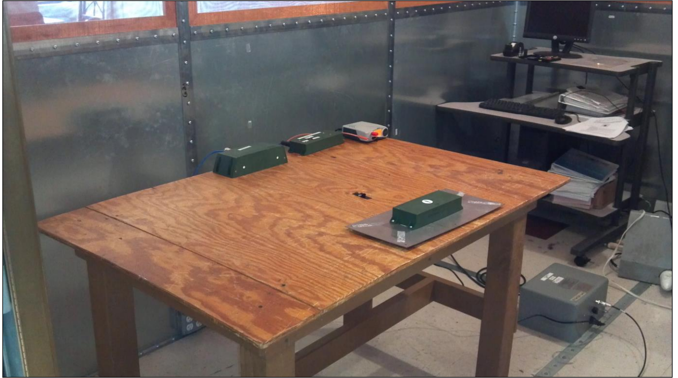
Photograph 1. Conducted Emissions, Test Setup
