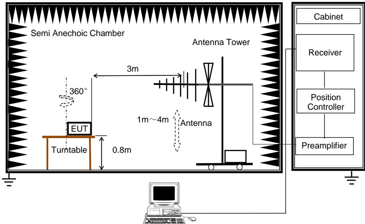
(b) Radiated Disturbance Test Set-Up Frequency above 1GHz
