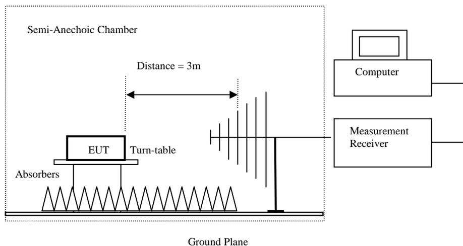
Absorbers placed on top of the ground plane are for measurements above 1000MHz only.
