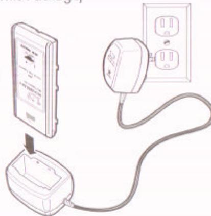
1. Insert the 7.2V NiCd rechargeable battery pack securely into the Battery Holder (as shown above).
