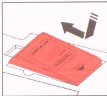
2. Turn compartment lock and slide the pack to release.
