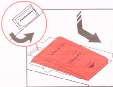
1. Slide supplied POWER CHARGE Battery into battery compartment and lock into place by turning compartment lock (as shown).
