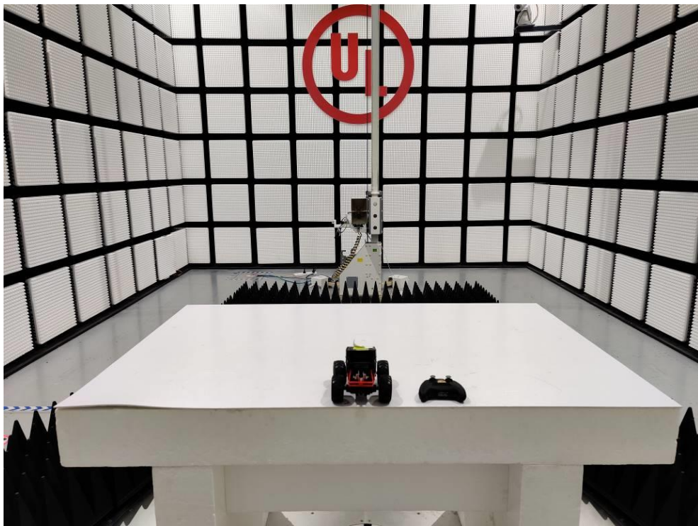
Radiated Emissions above 1GHz test setup photo
