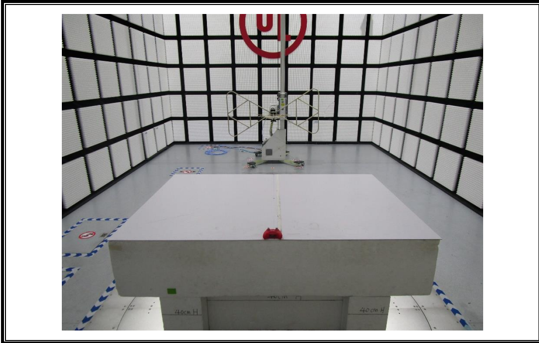
RADIATED RF MEASUREMENT SETUP (30MHz ~ 1 GHz)
