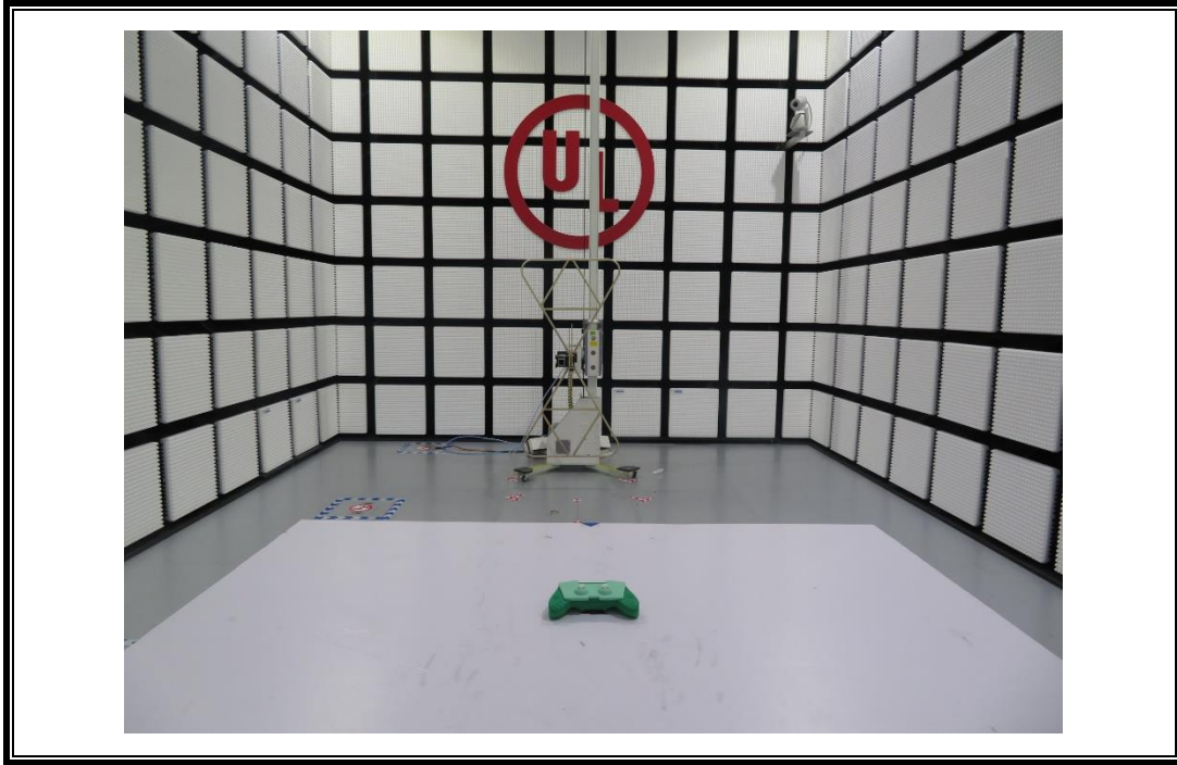
RADIATED RF MEASUREMENT SETUP (30MHz ~ 1 GHz)
