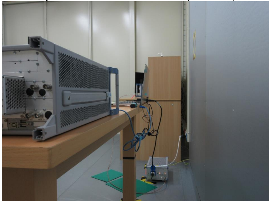
Photograph 8: Test Setup for Mains Conducted Emissions (Back View, BTM-510CC)
