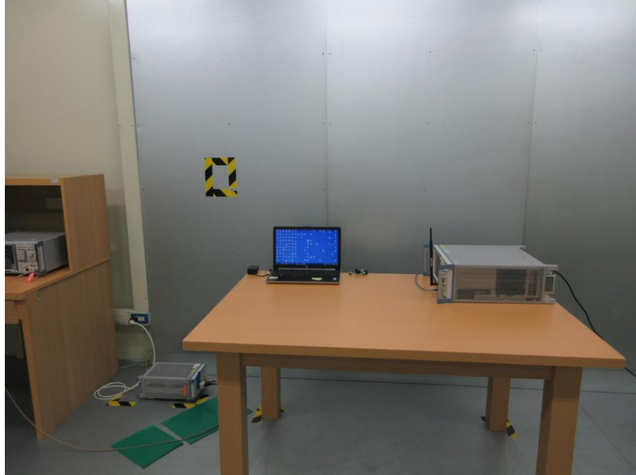
Photograph 7: Test Setup for Mains Conducted Emissions (Front View, BTM-510CC)
