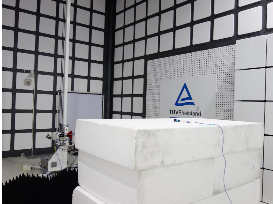
Photograph 3: Test Setup for Spurious Emissions (Back View 1, BTM-510CC)
