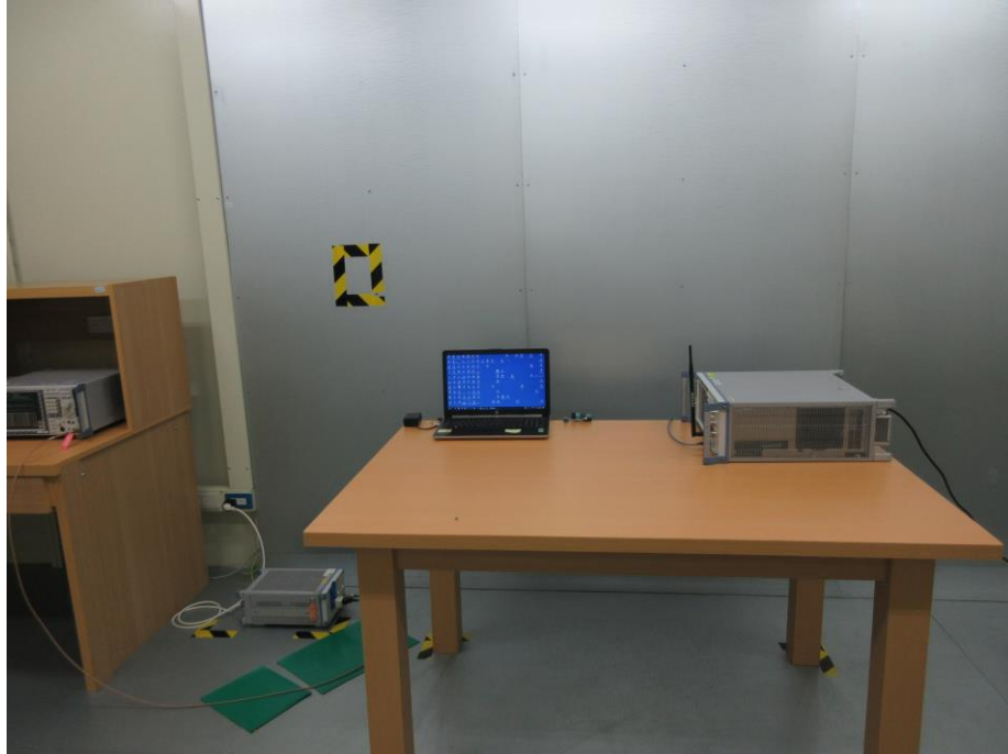
Photograph 15: Test Setup for Mains Conducted Emissions (Front View, BTM-510CD)
