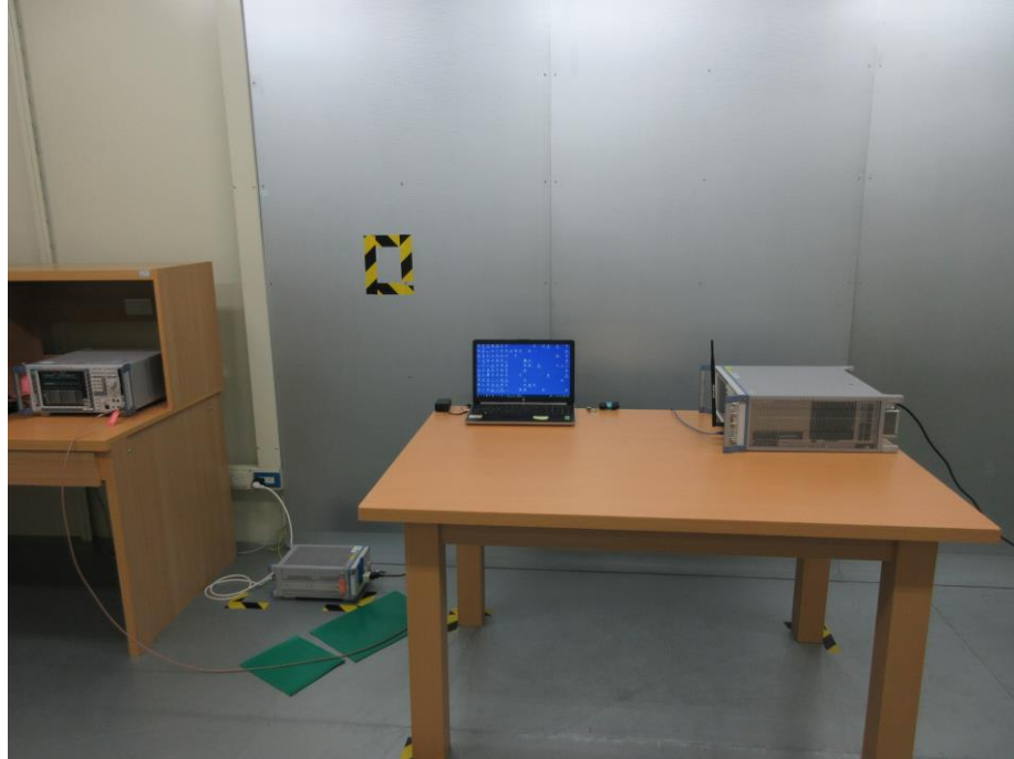
Photograph 23: Test Setup for Mains Conducted Emissions (Front View, BTM-510CR)
