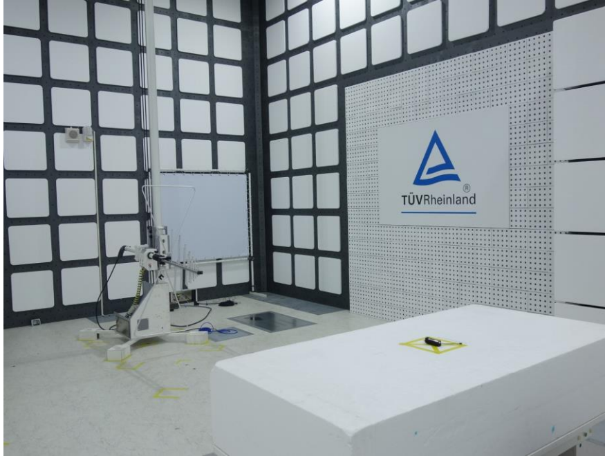
Photograph 3: Set-up for Spurious Emissions (Back View 1)
