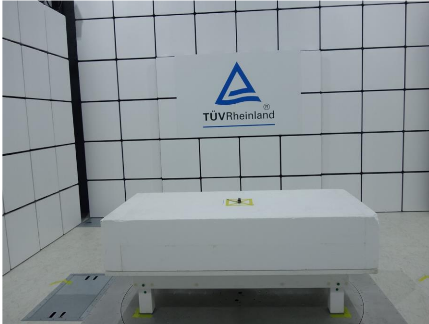
Photograph 1: Set-up for Spurious Emissions (Front View 1)
