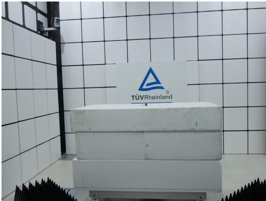
Photograph 2: Set-up for Spurious Emissions (Front View 2)
