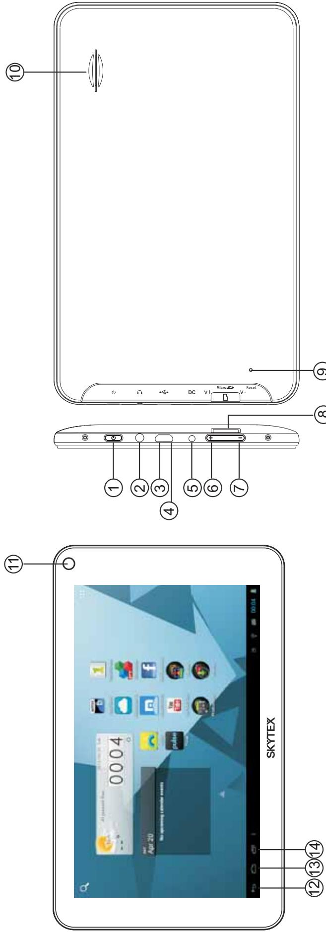
8. MicroSD Card Slot Load external storage memory card (up to an additional 32GB).
