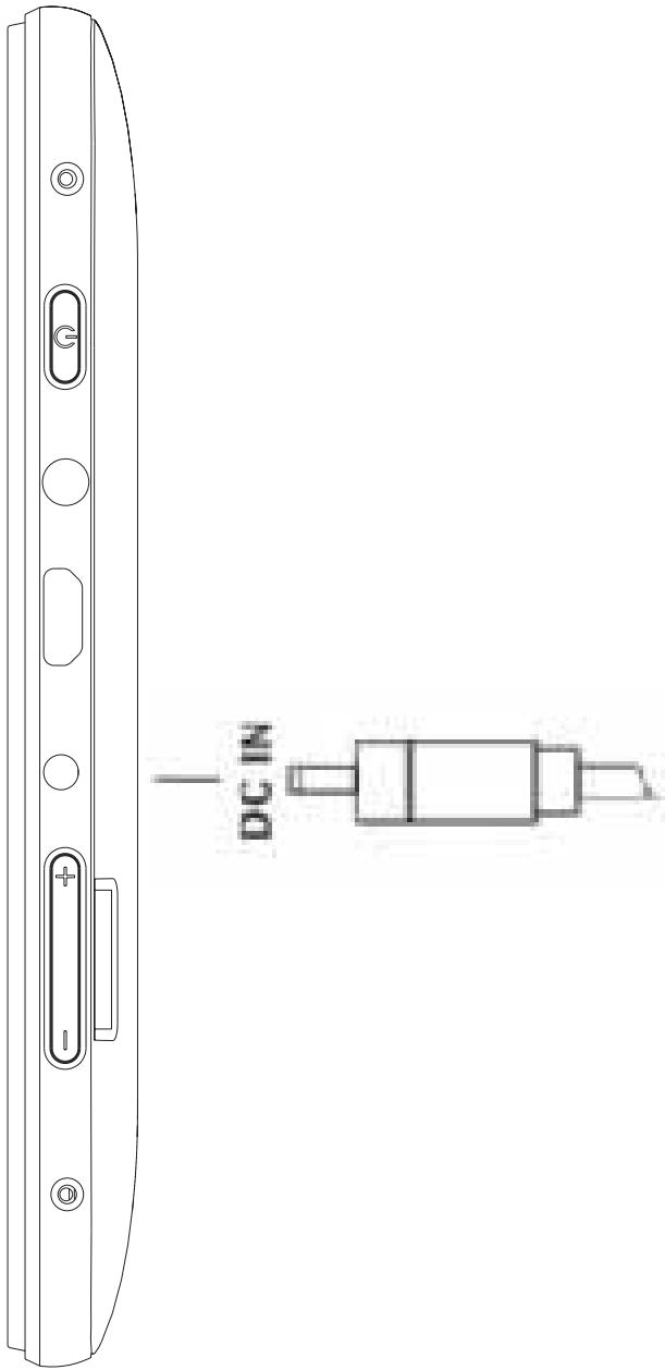
Note: When charging the Tablet while powered OFF, the battery indicator appears momentarily. Although the battery indicator disappears, the Tablet will continue to charge.
