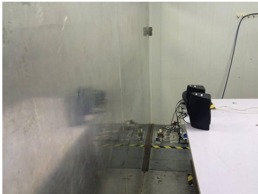
**RADIATED EMISSION TEST****Below 1GHz**
