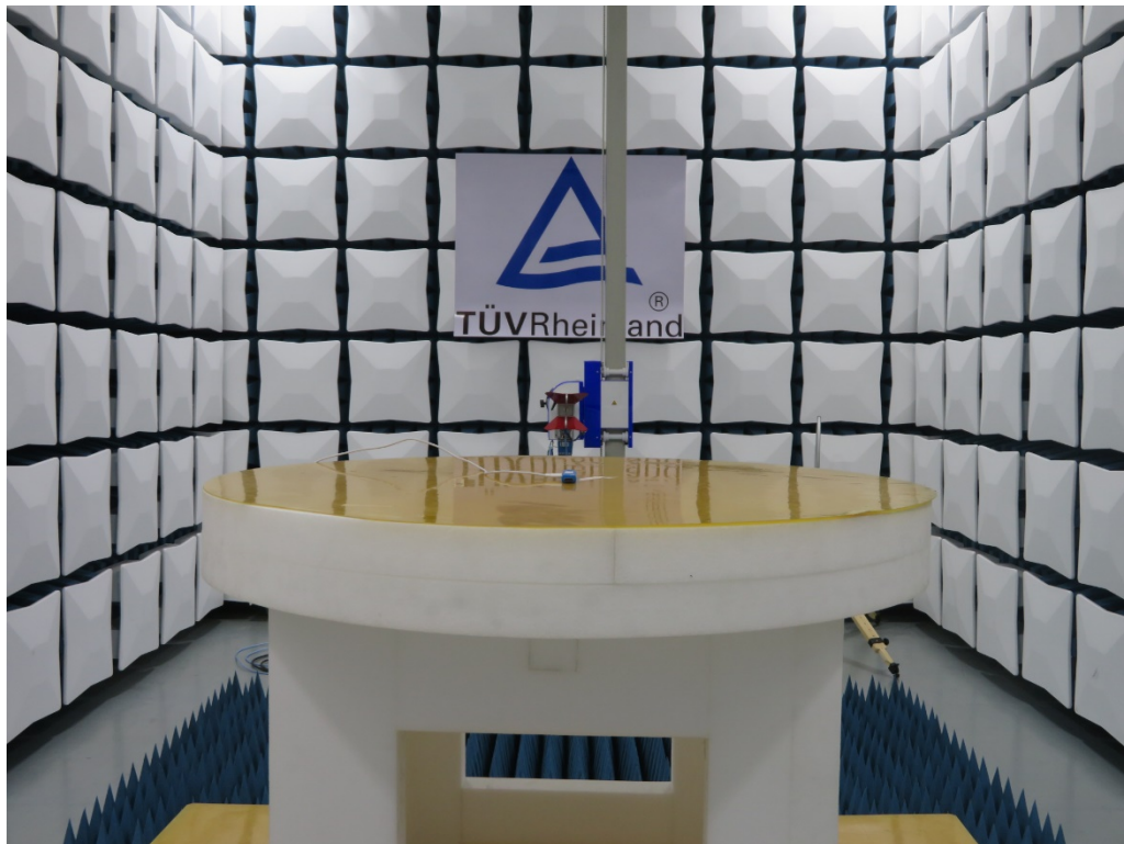
Photograph 2: Set-up for Radiated Spurious Emission, Above 1GHz
