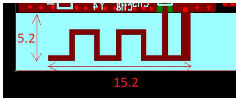
*Figure 1 Physical dimension (mm)*
