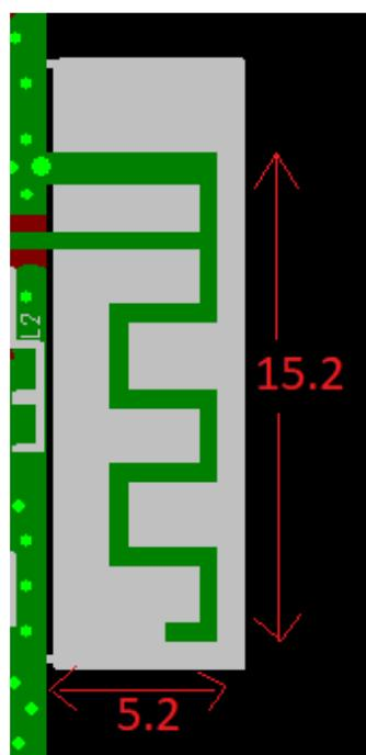
Figure 1 Physical dimension (mm)
