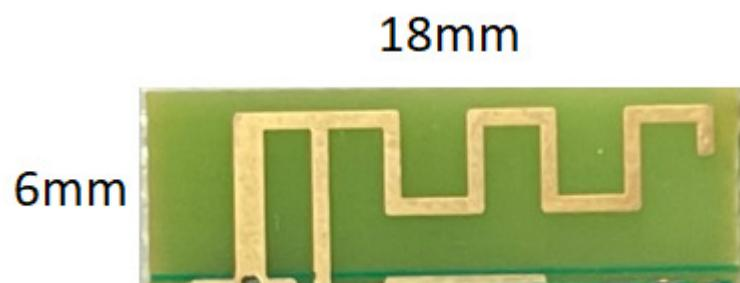
*Figure 1 Physical dimension (mm)*
